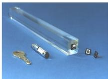
The crystals have a front face of about  $22 \times 22$  mm<sup>2</sup> — which matches well the Molière radius of 22 mm. To limit fluctuations on the longitudinal shower leakage of high-energy electrons and photons, the crystals must have a total thickness of 26 radiation lengths — corresponding to a crystal length of only 23 cm
