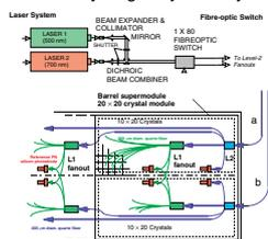
The light monitoring system, shown on the left, is designed to inject light pulses into each crystal to measure the optical transmission. The pulses are distributed via an optical-fiber system. The system is designed to continuously monitor the calorimeter
