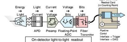
The first element is the  $PbWO_4$  crystal which converts energy into light. The light is converted into a photocurrent by the photodetector. The relatively low light yield of the crystal necessitates a preamplifier in order to convert the photocurrent into a voltage waveform. The signal is then acquired and digitized. The resulting data are transported off the detector via optical fibre to the upper-level readout
