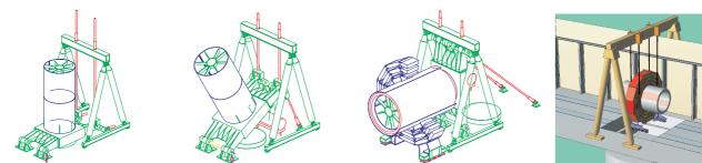
Rotation of the winded coil to horizontal position, sliding in the central yoke and lifting in the pit
