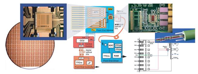
The system will provide analogue data from ~10 million channels of the microstrip tracker with minimal power and material. Electronic noise should be sufficiently low to ensure high efficiency and bunch crossing identification. Performance is ultimately limited by the speed and magnitude of detector signals and the radiation environment. Lifetime doses of 100kGy (10Mrad) and fluences of 2 x 10<sup>14</sup> hadrons cm<sup>-2</sup> are expected in the innermost layers
