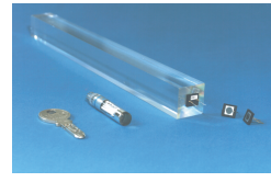
A full size (23cm long) lead tungstate crystal with a mounted APD
